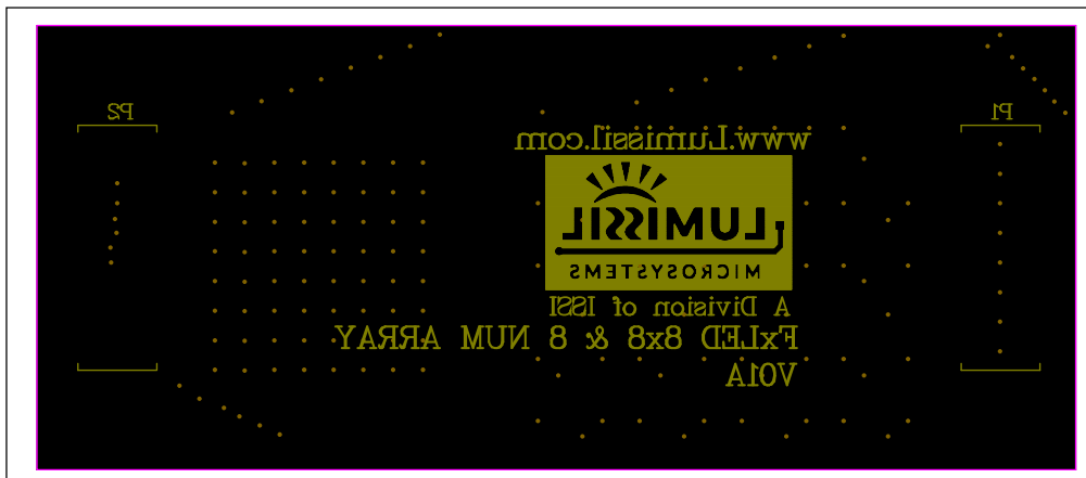
Figure 11: LED Board Component Placement Guide - Bottom Layer
