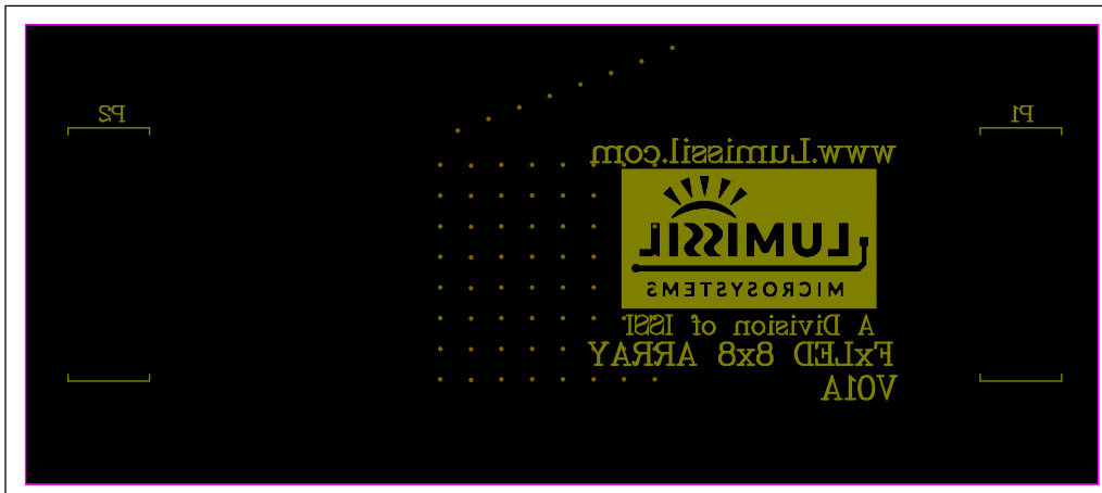
Figure 11: LED Board Component Placement Guide - Bottom Layer
